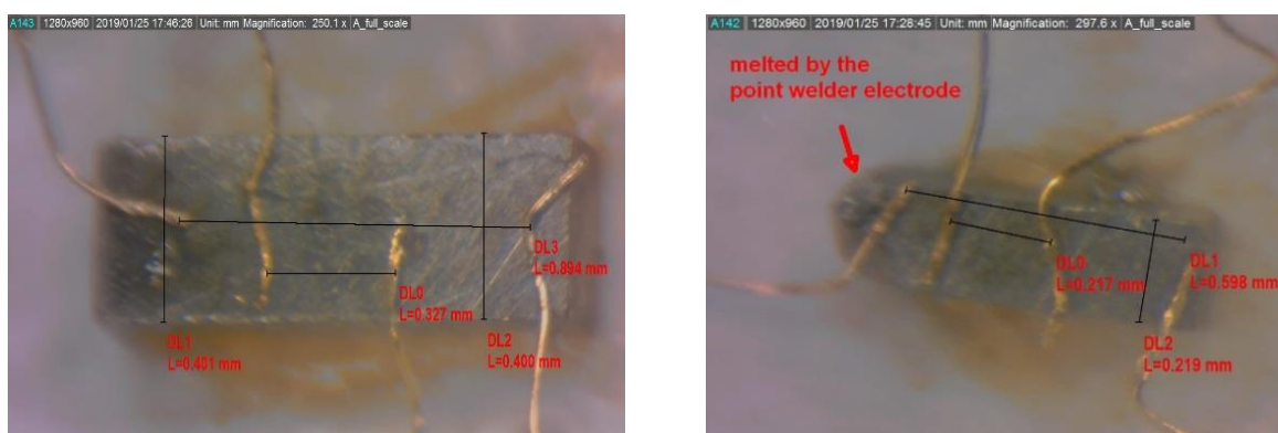
Fig. 1. Single crystals of U_2Ni_2Sn mounted for the resistivity measurement in the [001] (left) and [110] (right) direction.
