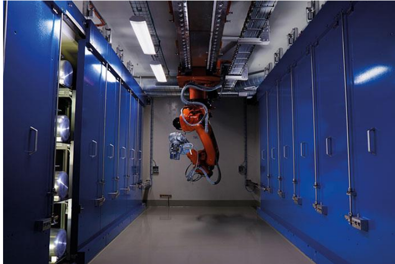
Fig. 2. Robot used in the production of radioisotopes for medicine at CERN.
