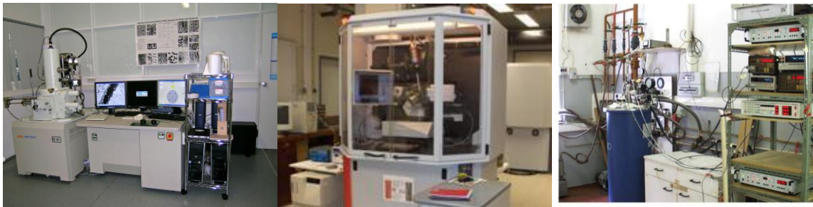
Fig. 3. a) FEG-SEM, b) single crystal X-ray diffractometer, c) electrical magneto-transport characterization facility.
