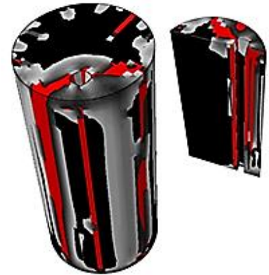
Figure 1: Crack pattern as a result of tensile strength excess at the point of steel's yielding initiation. Massive cracks are shown in red colour.
