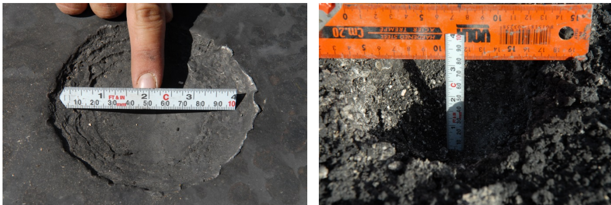
Fig. 2: Craters remained following detonation of the same charge on different surfaces types: Steel (clean) on the left and Asphalt (dirty) on the right.
