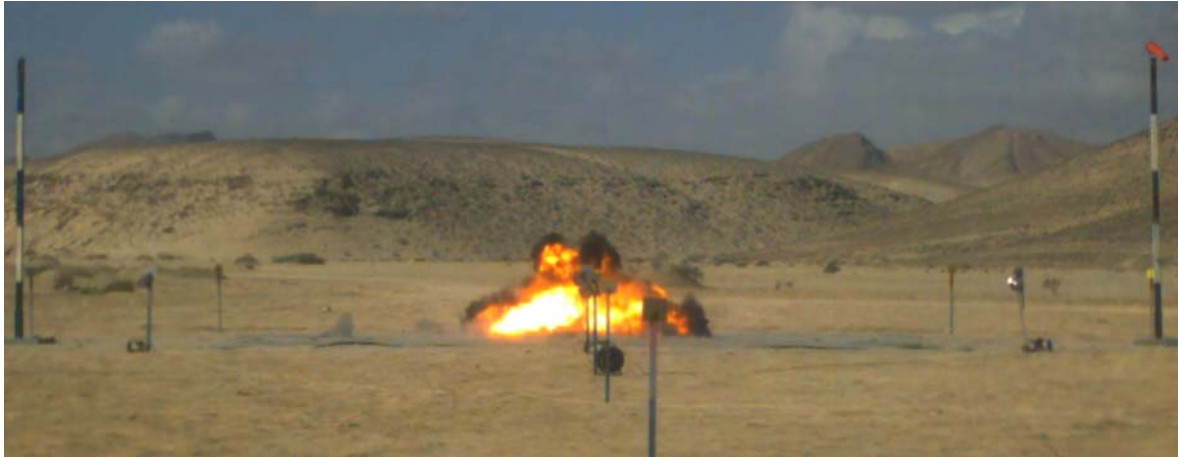
Figure 1: Fireball snapshot of 0.25 kg (TNT) during the afterburn stage at t=28.3 ms.
