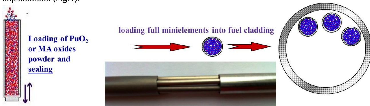
Fig.1 Scheme of loading of \text{PuO}_2 or MA oxides powder and minielements into fuel cladding.
