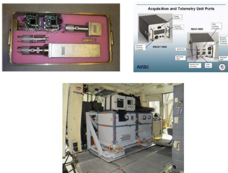
Figure 1. Interior of the SPARCS-A pod and The SPARCS ATU connections, up. The Air ram2000, down.
