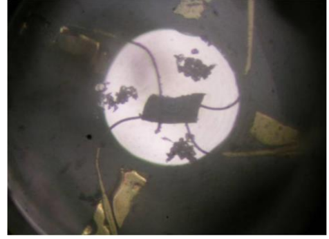
Fig. 4 Photograph of the sample with four electrodes and Ruby in loaded diamond-anvil cell.
