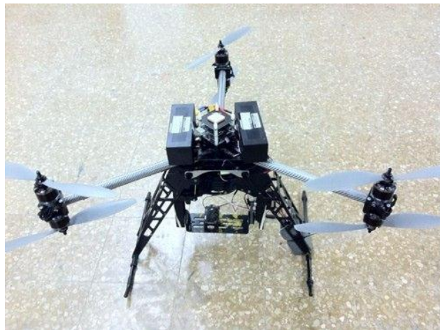
Figure 1. The Mikro-kopter with its batteries and six electric propellers. A small camera is located as is payload.
