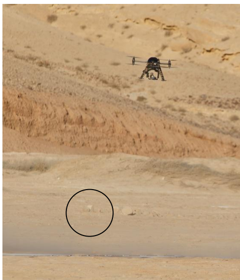
Figure 2. The Mikro-kopter measuring the radioactive field of hidden source.
