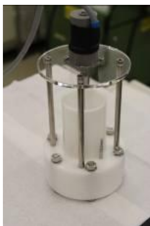
Figure 3. Picture of the molecular plating cell used to prepare thin 235 U layers on Al foil.
