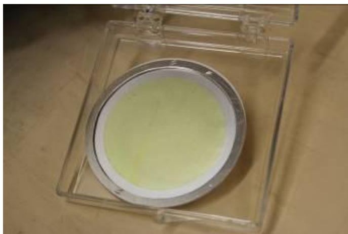
Figure 2. Thin 235 U layer prepared by molecular plating on a thin Al foil.
