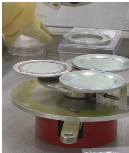
Figure 1. Rotating system holding the backings with the vacuum deposited ^{235}\text{UF}_4 layers and the masks.
