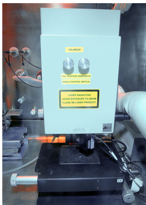
Fig. 1. Glovebox-Housed Raman Probe for Actinide Compound Analysis
